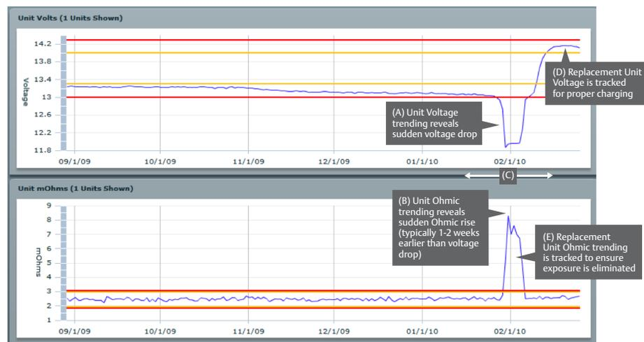
Figure 2: Battery Failure caused by Sudden Impedance/Resistance Rise
